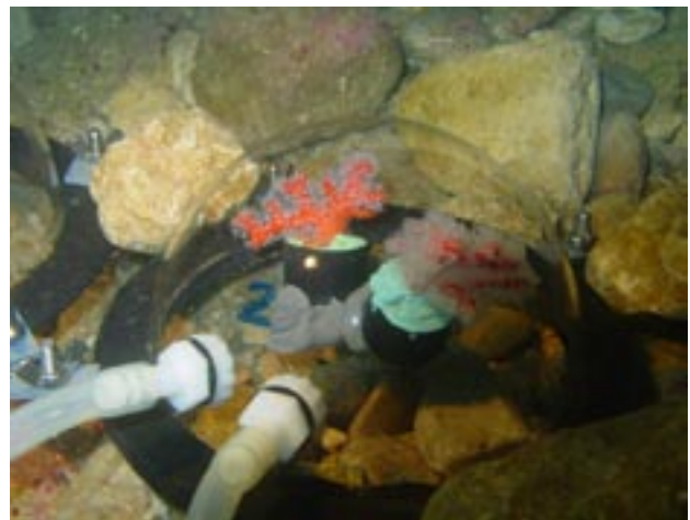
Figure 2: Two red coral colonies in an in situ incubation chamber which is connected to a portable submersible pump (not shown).
