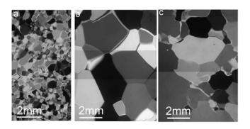
**Fig. 5.** Composite photomicrographs taken between crossed polarizers. (a) Initial sample. (b, c) After 3 days at  $-4.9^{\circ}$ C: annealing only (b); creep test at 0.52 MPa and 3.58% total strain (c).
