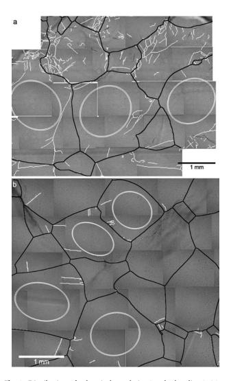
**Fig. 9.** Distribution of subgrain boundaries (marked as lines). Most subgrain boundaries are attached or close to a grain boundary (black), forming a subgrain-boundary-free core (approximately indicated by ellipses), which is not sharply defined. (a) Horizontal section (-4.8°C, 0.35 MPa, 1.22% total strain). (b) Horizontal section (-4.9°C, 0.35 MPa, 0.44% total strain). Note: Distribution inside grain is highly heterogeneous, e.g. areas of higher subgrain-boundary density (top of (a)).
