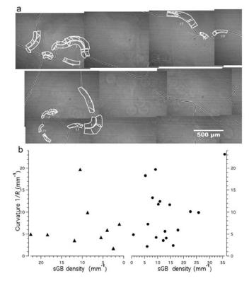
**Fig. 10.** Subgrain-boundary density in the vicinity of curved grain boundaries ( $-4.8^{\circ}$ C, 0.52 MPa, 8.56% total strain). (a) Schematic showing how subgrain-boundary density was determined with measured areas, subgrain boundaries and curvatures. Numbers refer to the measurement. (b) Curvatures against subgrain-boundary densities. Areas on convex ( $\bullet$ ) and concave ( $\blacktriangle$ ) sides of the curve are shown separately.
