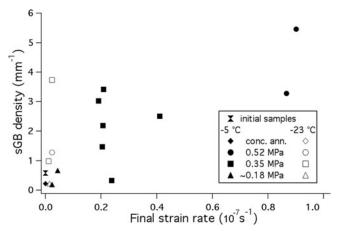
Fig. 6. Mean subgrain-boundary density against final strain rate. Mean over four to six selected regions (area:  $\sim 5 \text{ mm} \times 6 \text{ mm}$ ) in a section. Further experiments are required.
