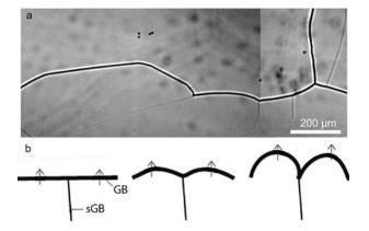
**Fig. 12.** Extensive interaction of subgrain boundaries with grain boundaries. (a) The geometry indicates pinning of a moving grain boundary by the subgrain boundary (–4.5°C, 0.35 MPa, 2.8% total strain). (b) Conceptual model; the grain boundary is moving towards the top of the picture (arrows indicate direction of movement) and the subgrain boundary pins it where they meet, in a similar way to particle-pinning of grain boundaries.
