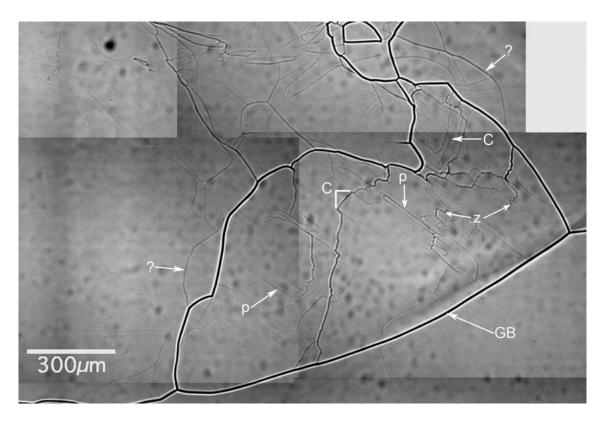
Fig. 7. Types of subgrain boundaries in a vertical section ( $-4.8^{\circ}$ C, 0.52 MPa, 8.56% total strain). GB – grain boundary; p – parallel subgrain boundary; ? – not yet classified subgrain boundary; c – classical polygonization type subgrain boundary.
