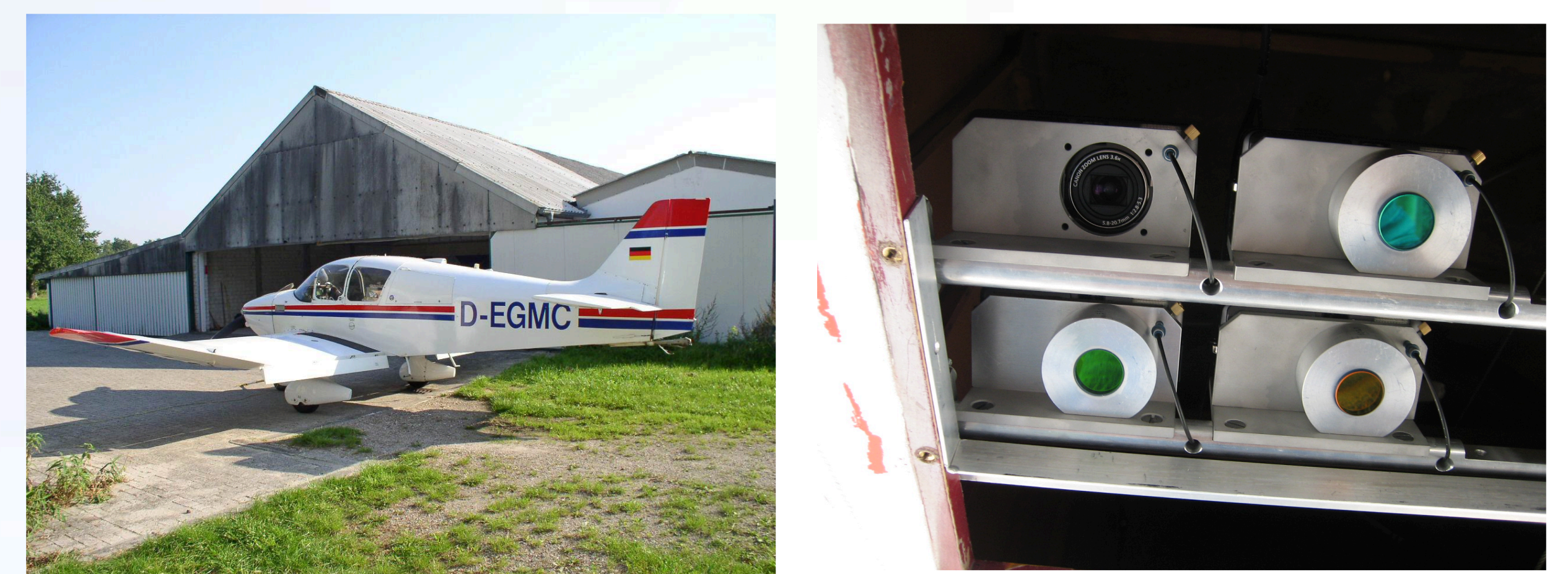
Fig. 2: Left: The airplane. Right: The four cameras mounted to the bottom hatch of the airplane, three having interference filters.
