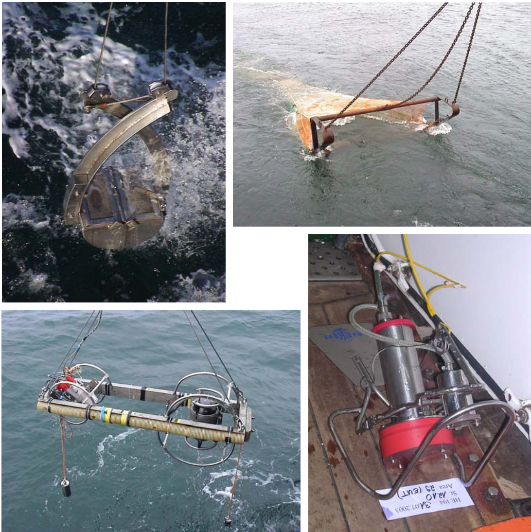
Figure 8: Main sampling gears used in this thesis: van Veen grab (upper left), beam-trawl (upper right), photo swing (lower left) and video camera (lower right).
