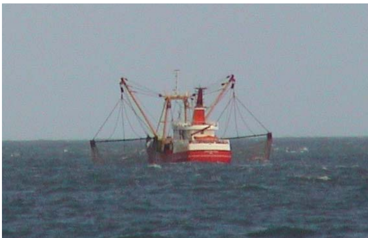
Figure 2: Modern beam trawler with a 12 meter beam trawl at either side, typical of the study area.
