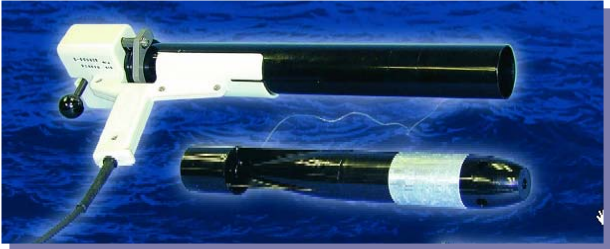
Fig. 2: XBT Hand Launcher ( www.sippican.com )
