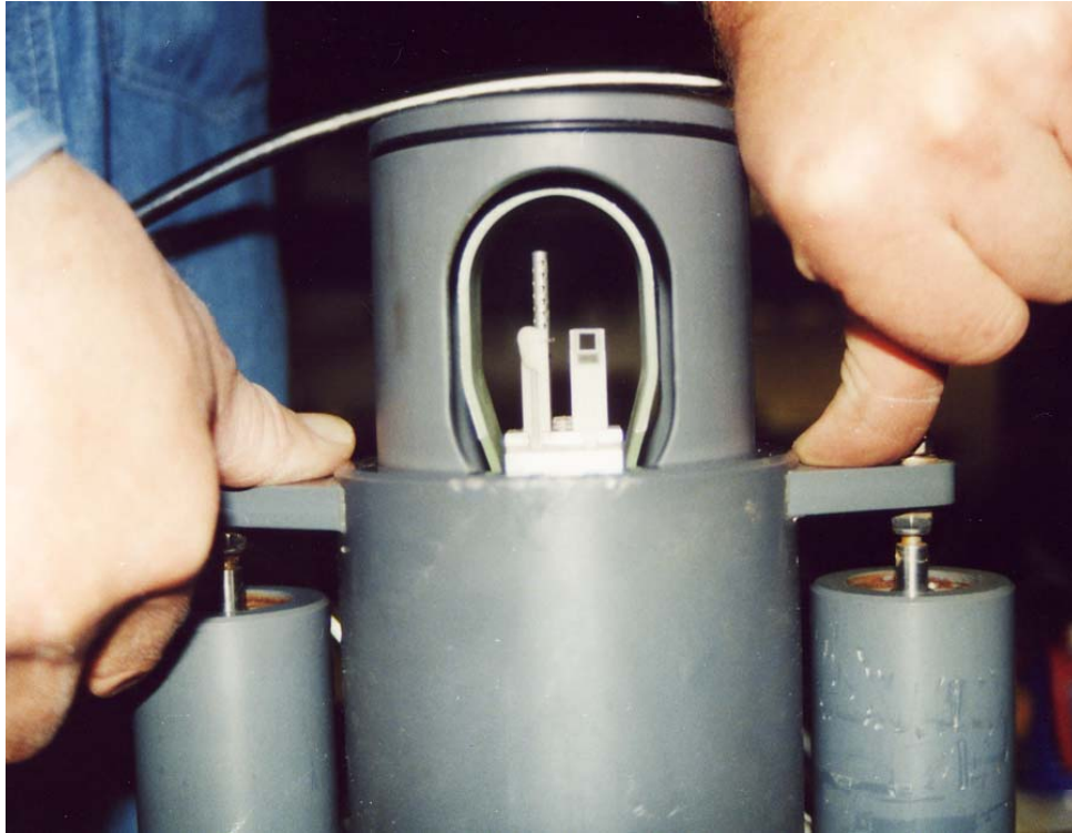
Fig. 5: Cold cover mounted at Mark IIIB CTD. Water pressure greater than 5 dbar forced the housing in the open position which was done here manually by pushing down the pressure releases.
