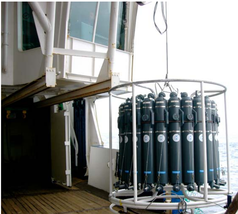
Fig. 3: 24 bottle water sampler; 12 liter size each. The instrument shown here is a SBE32 Carousel. The CTD SBE911plus is mounted vertical behind the bottles.
