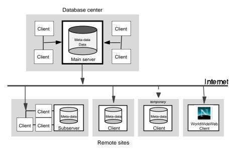
Network concept of the PANGAEA system. Data are accessible from the main server via the Internet by specific clients which allow the import of data and have a high functionality. General access on published data is provided through WWW clients.
