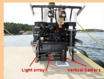
Fig 5) ROV used in collection of video data from Tisler reef for mosaicing.
