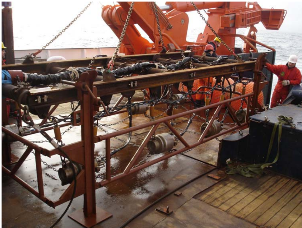
Fig. 3.3: G.Gun™ cluster used as seismic source
