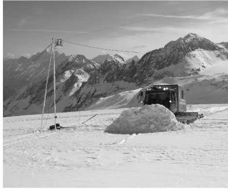
Figure 3.11.: The creation of the artificial avalanche mound above the phantom body.
