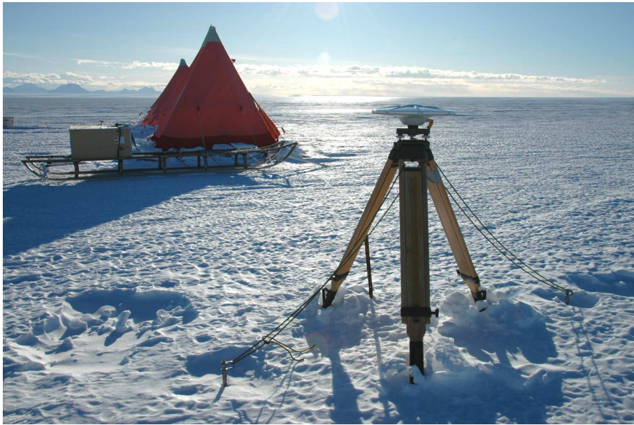
Figure 3.2.: Setup of GPS reference station on ice (field camp U9).
