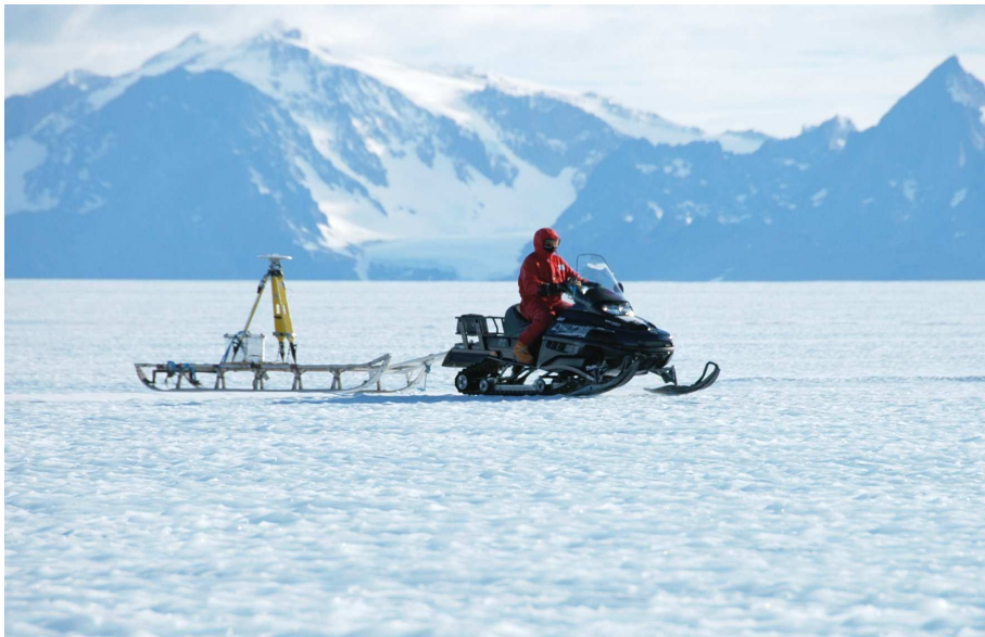
Figure 3.3.: Setup of kinematic GPS observations. A GNSS antenna (TRM57971.00) is mounted on a tripod on a Nansen sledge. The aluminium box on the sledge houses the TRIMBLE R7 GNSS receiver and the battery. The sledge is pulled by a two-stroke Lynx Yeti 550 snow mobile.
