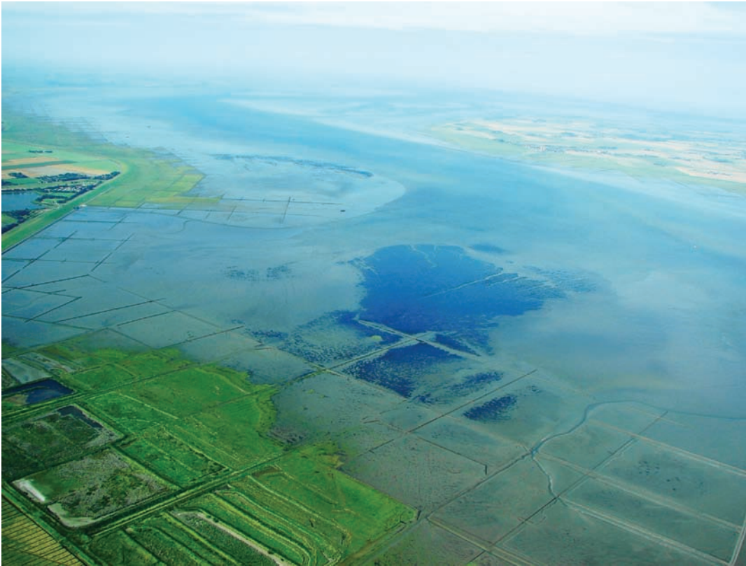
Figure 4.8: Well integrated management is required to meet multiple targets. The salt marsh (lower left) has received dredged sediment from an adjacent harbour site which is silting up. Construction of brushwood groynes for land claim disturb a seagrass bed (dark patch in centre), and in the shelter of these groynes, the introduced Spartina -grass is spreading into the mud flat. Protecting natural values at such a shore will be a growing challenge when sea level rise accelerates in the coming decades (Photo: K. Reise).
