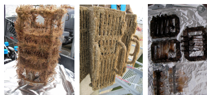
Fig. 4 Biofouling affecting the different sampling cages (left, middle) as well as the different tested passive samplers (silicone rubber sheets and LDPE membranes)
