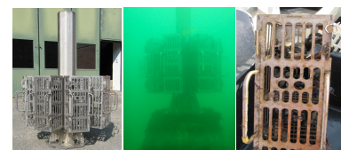
Fig. 3 Titanium sampling cage for deployment of preconditioned mussel cultures; cage shown before, during and after deployment
