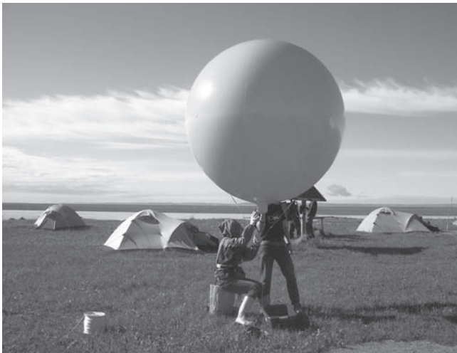
Figure 4. Tethered balloon, filled with helium, diameter 2–3 m.
