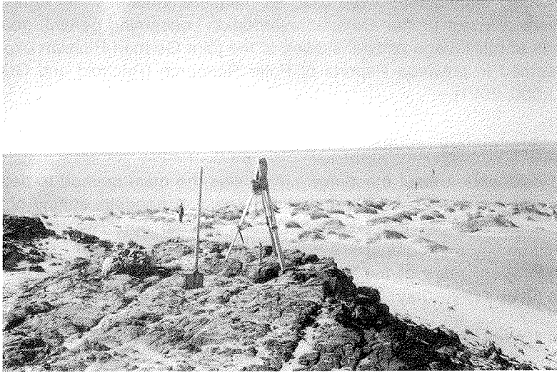
Figure 7-2: Theodolite survey of the Northern Cape of Babaryna Island and vast wind affected mud flat (barrier islands are on the remote edge of the flat), August, 2001.
