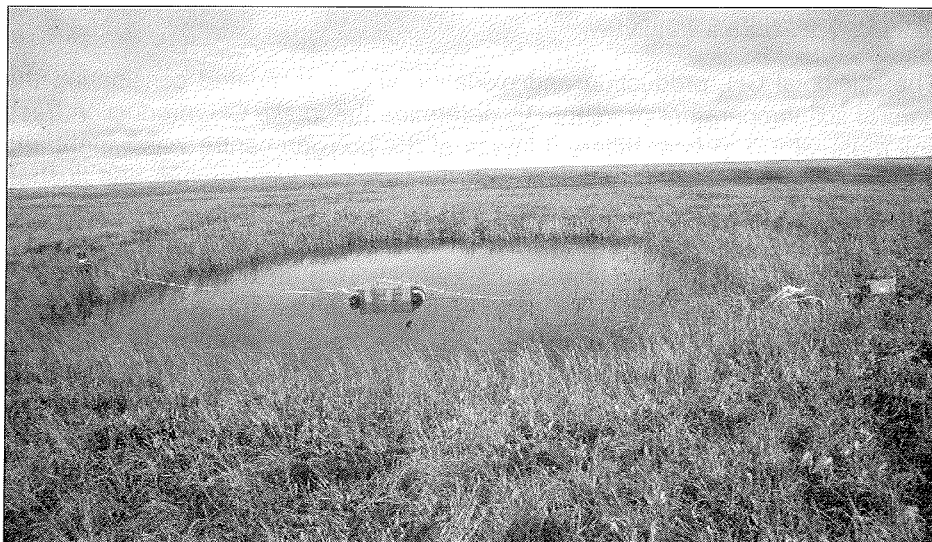
Figure 3-5: The polygon lake with the floating chamber in the middle of the lake.
