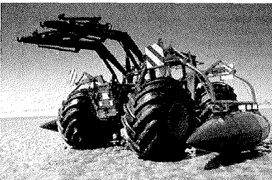
Fig. 5a/b. Service tractor. (a) Tractor with hydraulic arms and large, wide wheels to minimize pressure impact on the Wadden Sea bottom. (b) Tractor in action for transport and placement of bags.
