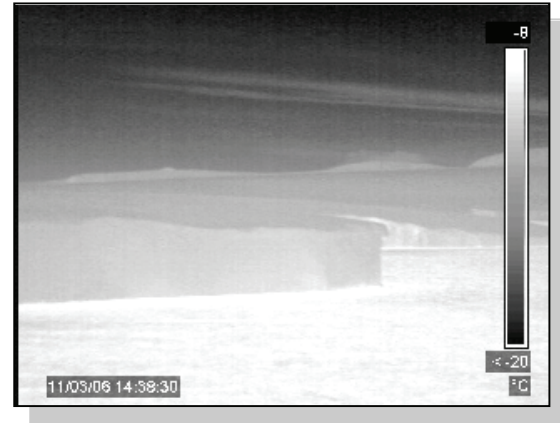
Fig. 14.5: The same scene as in Pic 4 from the IR camera using a 12 degree telephoto lens with a better resolution of the landscape
