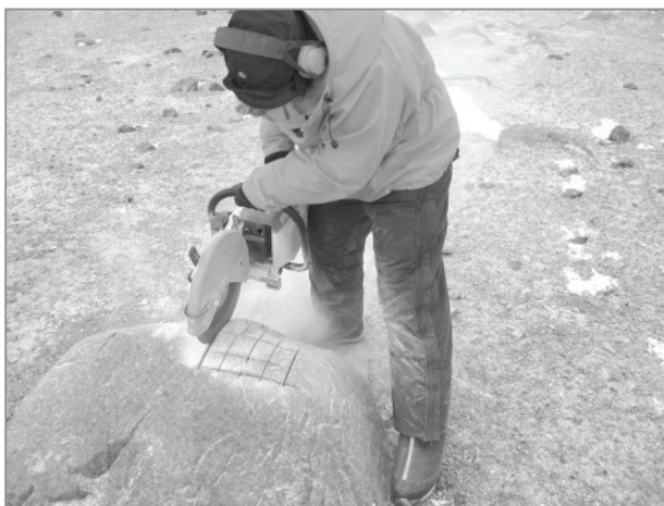
Fig. 9.3: Petrol-powered cut-off saw in use on granite boulder on the un-named island west of Canisteo Peninsula
