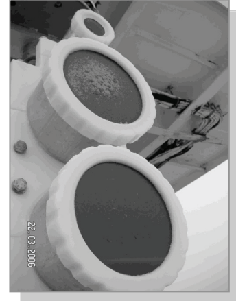
Fig. 14.3: Three cameras - visual, infrared 12 degree and infrared 7 degree (up to down).
