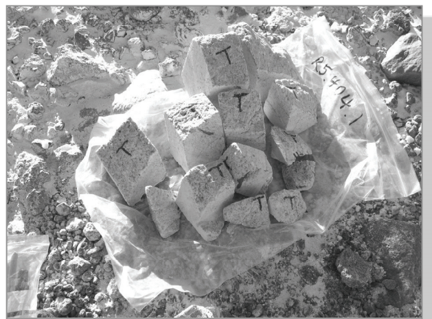
Fig. 9.4: Granite blocks removed using the Stihl saw and then a hammer and chisel. 'T' marks the upper surface of each block.
