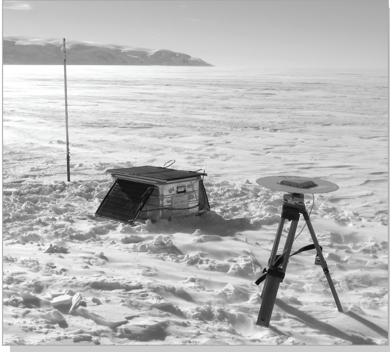
Fig. 10.3: Setup of the GPS station on Crosson Ice Shelf as an example for the stations on ice
