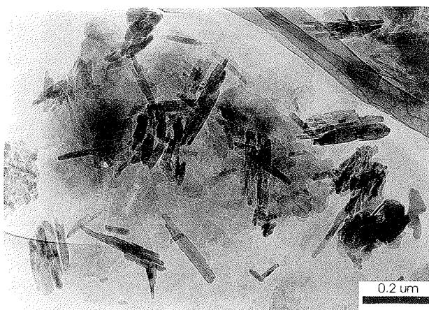
Fig. 9 - Core level 901.2 mbsf, TEM image showing smectite and Fe-oxides.
