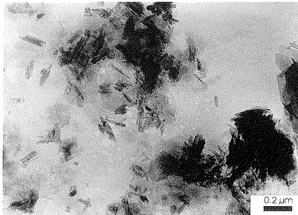
Fig. 11 - Core level 919.06 mbsf, TEM image showing aluminous smectites and Fe-oxides.
