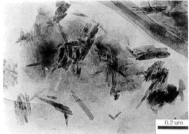
Fig. 12 - Core level 918.53 mbsf, TEM image showing aluminous smectites and kaolinites.
