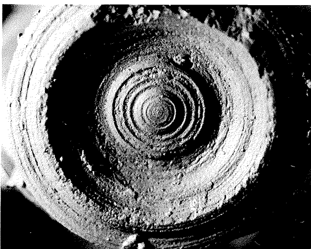
Fig. 14 - Photograph of the surface of a typical drilling-induced, horizontal fracture that developed near the base of the CRP-1 core (144.2 mbsf). The core was broken and spun due to sea swell-induced vertical motion of the drill bit, resulting in the finely etched circular grooves and striae. Core is 6.1 cm in diameter.
