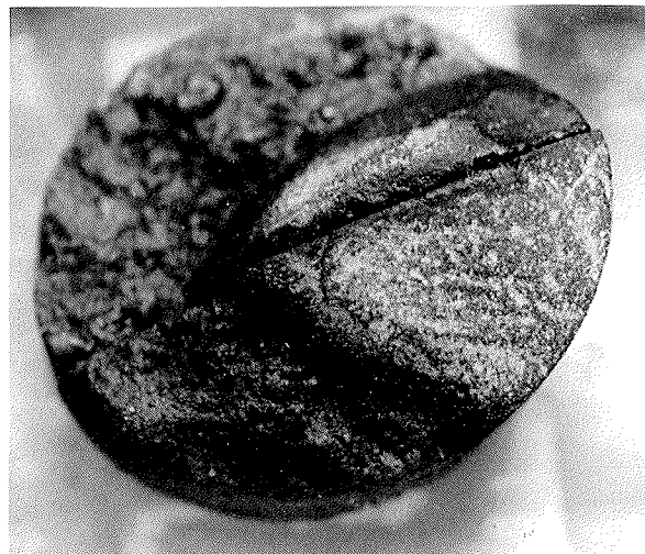
Fig. 3.14 - Striated mudstone clast from 738.40-738.42 mbsf. Core is 45 mm in diameter.
