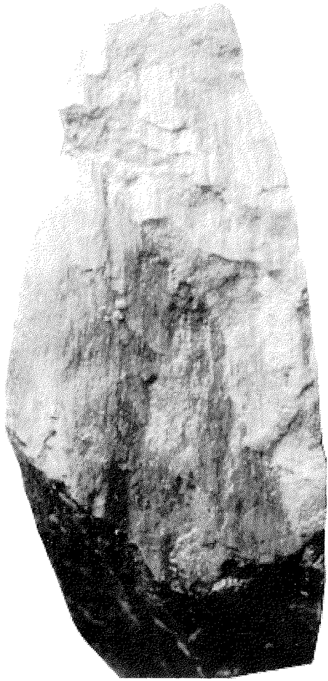
Fig. 2.5 - Slickensided microfault surface showing dip-slip motion in Oligocene strata, 407.81-407.90 mbsf. Core is 45 mm in diameter.
