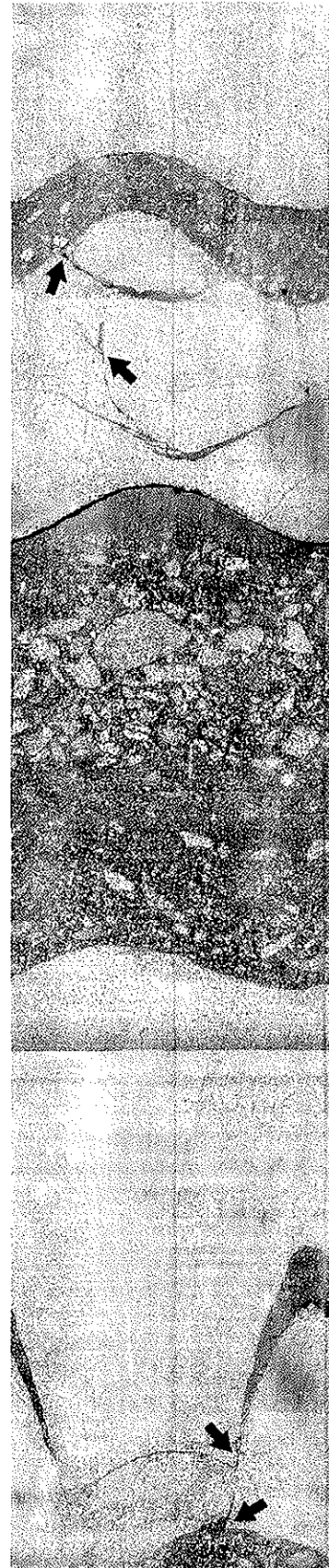
Fig. 2.9 - Fragmental bands in fault zone from 790-801 mbsf interpreted to form by cataclasis. Unrolled whole-core scan of 45-mm-diameter core between c. 794.10 and 794.74 mbsf. Note planar zones of fragmental material with moderate to steep dips and dark bands of injected material connecting them (arrows).
