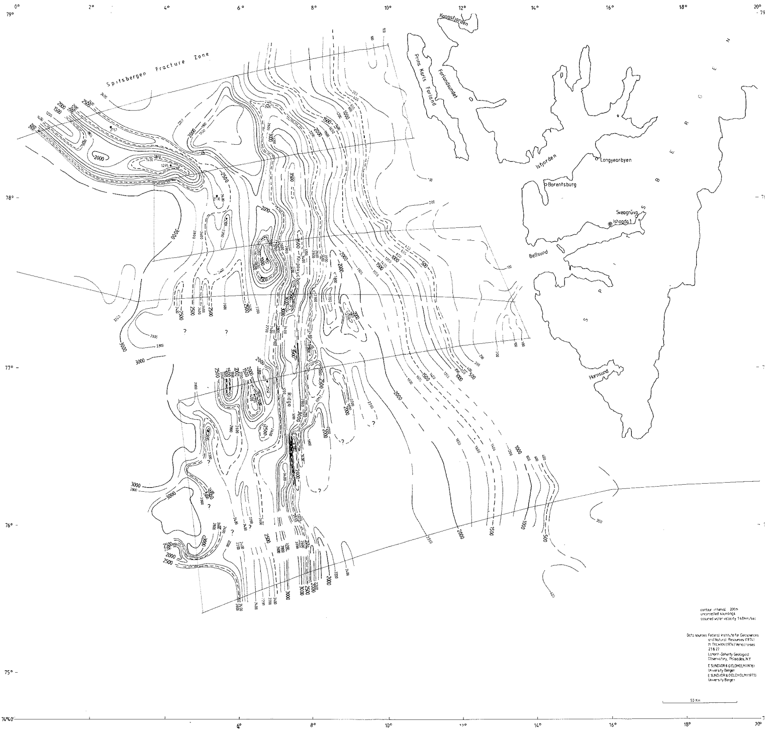
Fig. 2: Bathymetric map; contours are in meters using a nominal sound velocity of 1480 m/sec. Data sources: Lamont-Doherty Geological Observatory, Palisades, N. Y. (1966, 1969—70); Seismological Observatory, Bergen (1975—76); Federal Institute for Geosciences and Natural Resources (BGR), Hannover (1974).
