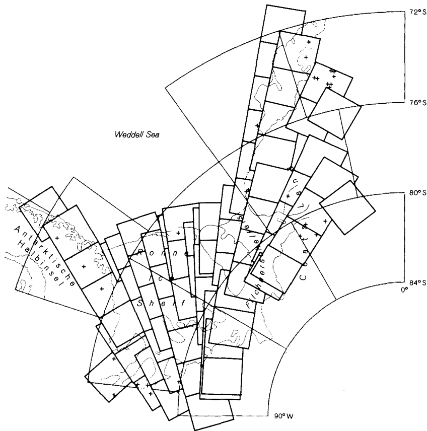
Fig. 5: Imagery coverage diagram of Landsat MSS mosaic "Filchner-Ronne-Schelfeis, Coats Land". + geodetic control by GPS or Doppler satellite positioning; map sheet line system based on International Map of the World 1:1.000.000.
