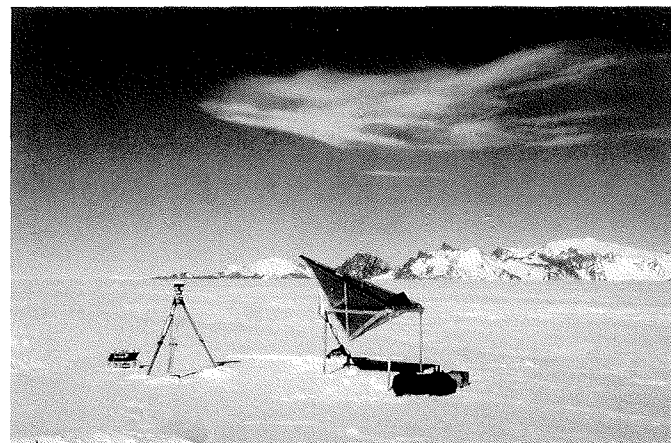
Fig. 2: Corner reflector on inland ice. The mountains in the background are part of the Wohlthatmassiv.
