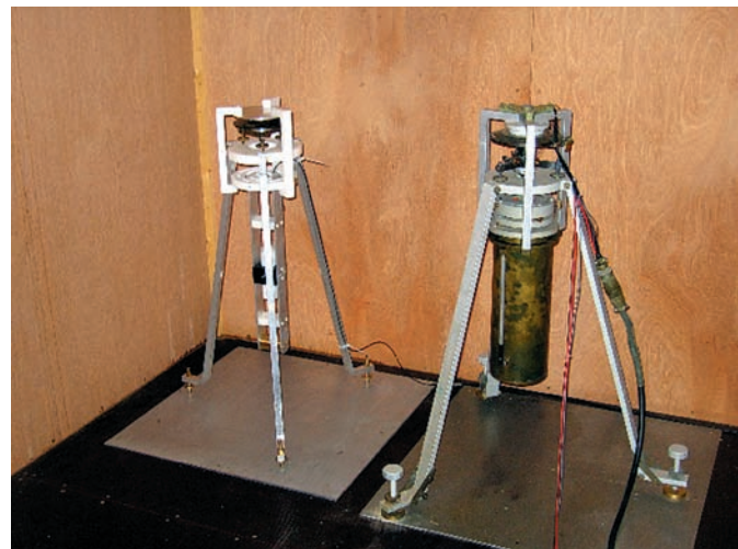
Fig. 5: The two 3-component flux-gate sensor systems inside the magnetic observatory for measuring the NS, EW and vertical component of the Earth's magnetic field. On the right side is the old system and on the left side the new system, which is now continuously operating since May 2006. Both systems are mounted on a cardanic suspension to avoid any tilt. Analogous and digital signals are transmitted by cable to the I27DE container for recording.
