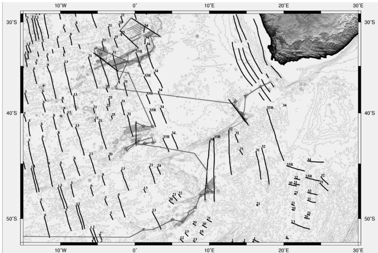
Fig. 5.1: The grey lines indicate the ship track. Magnetic isochrones are labelled 5-33R. The black lines with the magnetic flight pattern (dense grey lines) indicate the locations of the seismic refraction and reflection profiles across the Discovery and southernmost Cape Rise seamounts, as well as across the southern Walvis and Agulhas ridges.
