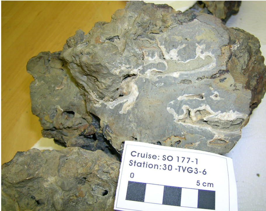
Fig. 5.4.3.11 Type 4-4: Huge irregular carbonate block, dark brown surface, porous with many protuberance in the size of 1-2.5cm dia., and many organisms living (corals, sponge, etc. shrimps) on the surface. Gray inside, micritic, aragonite precipitated inside some of the elongated voids, but no venting clams included. TVG 3
