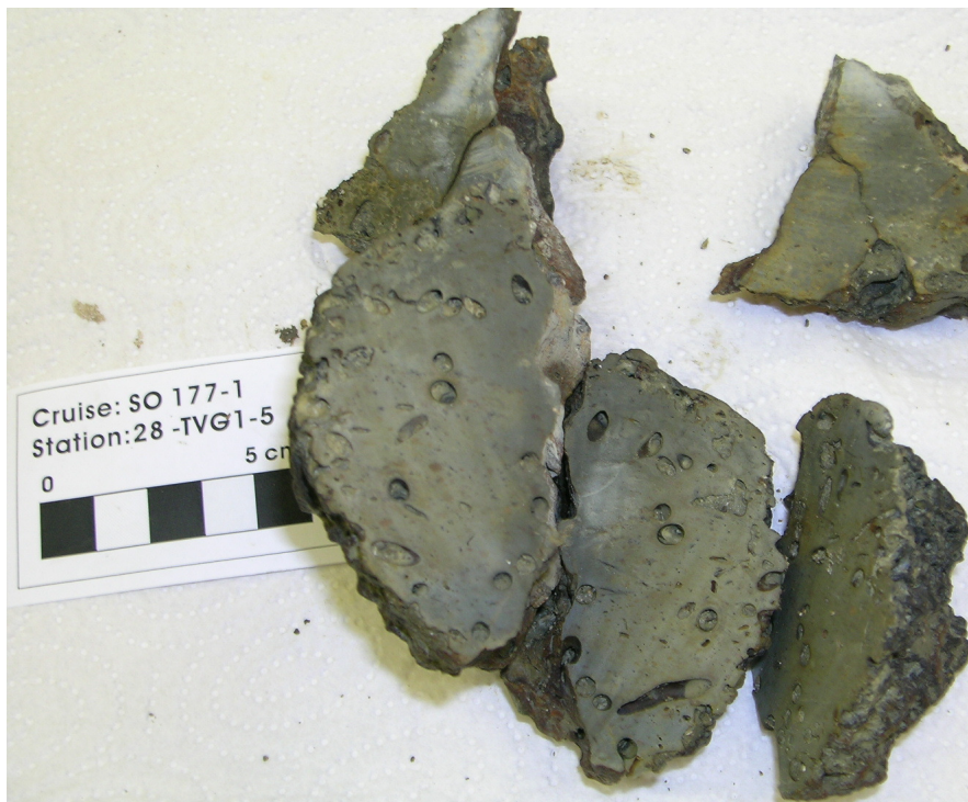
Fig. 5.4.3.3 Type 2: Seepage-associated concretion, massive, dark brown surface with Fe-Mn oxide coating and protuberances. Cross cutting shows that the inside is gray, micritic, abundant in holes with chitinous wall left by tube worms (2-5mm in dia. ), 12x8x4cm,TVG1
