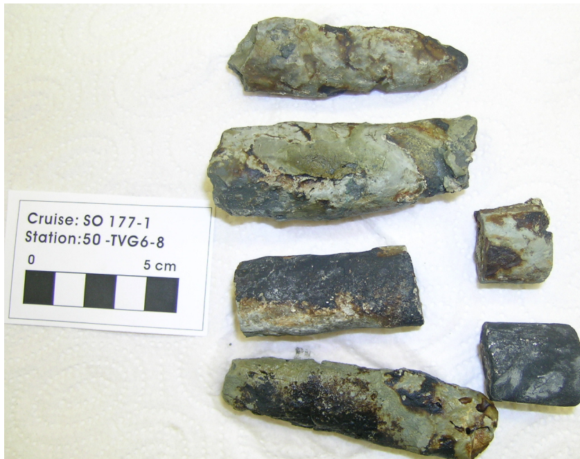
Fig. 5.4.3.8 Type 4-2: Tubular carbonaceous concretions, bullet like, 2.5cm in dia., cross section shows some samples have tube worm holes inside with chitinous walls. One sample has abundant pinholes. No apparent channel inside. TVG 6
