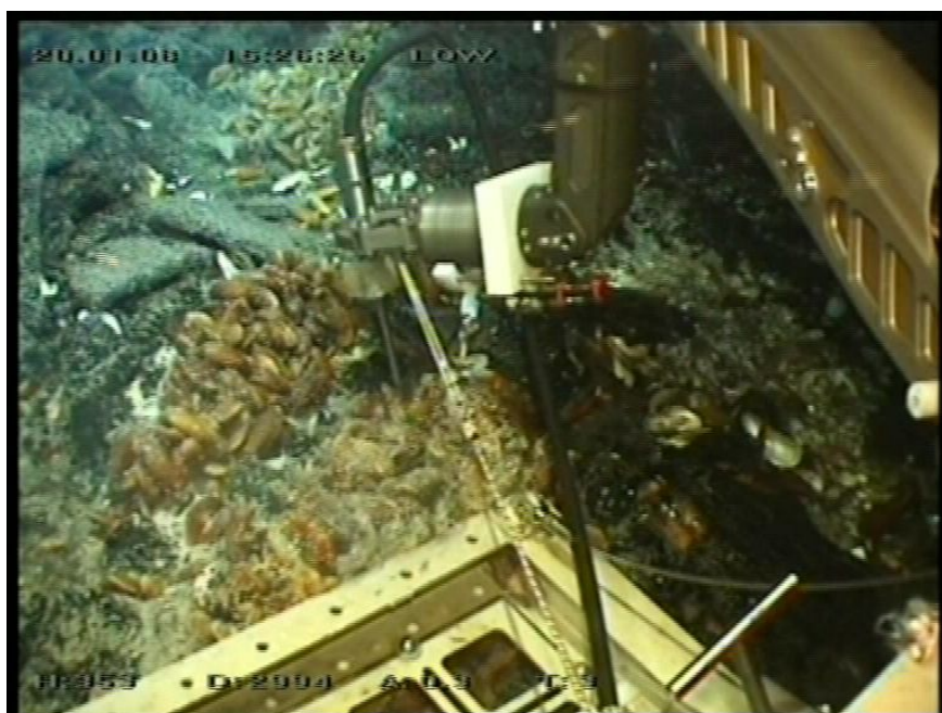
Fig. 2.4.3.6: Measurement of temperature with the 8-channel temperature logger at the low-temperature diffuse outlet at Clueless (52 ROV10).
