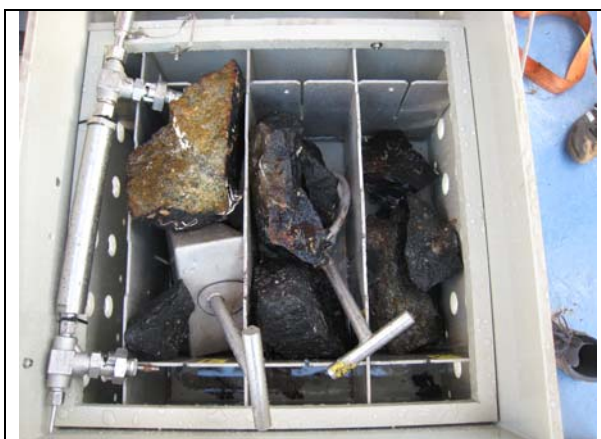
Fig. 2.4.10.5: The ROV drawer, configured for – and filled with – rocks. Bookkeeping required! Additional tools from left: IB sampler, shovel, bionet.
