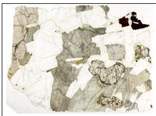
Fig. 2.4.10.8: View in plane polarized light of an entire thin section (3 cm long) showing olivine gabbro-norite. Sample D2-S12 from the 5°S core complex.
