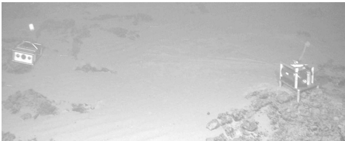
Fig. 2.10: OBP (left) and OBT (right) deployed at their final positions west of IRINA II.
