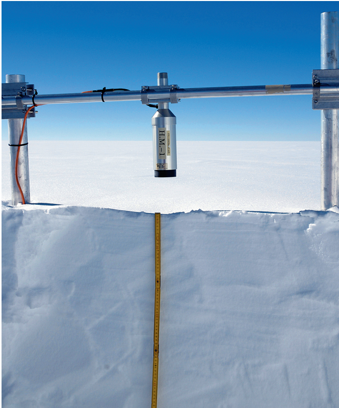
Fig. 28: Snow height ranger (ultra sonic) HM1 on the day of dismantling (23 Jan 2008). HM1 was operated by University of Utrecht. (Photo H. Oerter).
