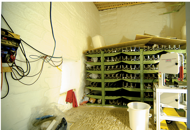
Fig. 18: View into the core buffer after drilling operation was finished. The shelf with the core troughs was used for temporary core storage, especially when drilling the so-called brittle zone to allow the cores to get adjusted to the temperature and air pressure in the science trench. On the left, the entrance to the ice cave for the investigation of physical properties is visible. (Photo H. Oerter, 29.01.2008).
