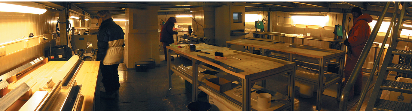
Fig. 22: View into the cold lab of AWI at Bremerhaven, where ice-core processing of the EDML core took place. Processing – at an average temperature of -20^{\circ}\text{C} – starts on the left side, where the cores are cut by the horizontal saw. For the cuts perpendicular to the core axis several other saws, e.g. on the right side, are available in the cold lab. In the middle of the room the cores are scanned on a bench with a moving line-scan camera. (Photo H. Oerter).
