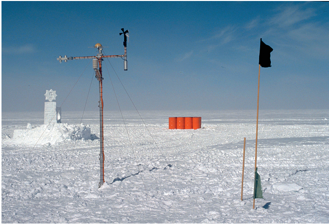
Fig. 25: The automatic weather station, AWS9, at site DML05 after construction on December 31, 1997. AWS9 was operated at this location until January 2001 and then shifted approximately 150 m to the NNE (Fig. 26). AWS9 belongs to University of Utrecht. (Photo H. Oerter).
