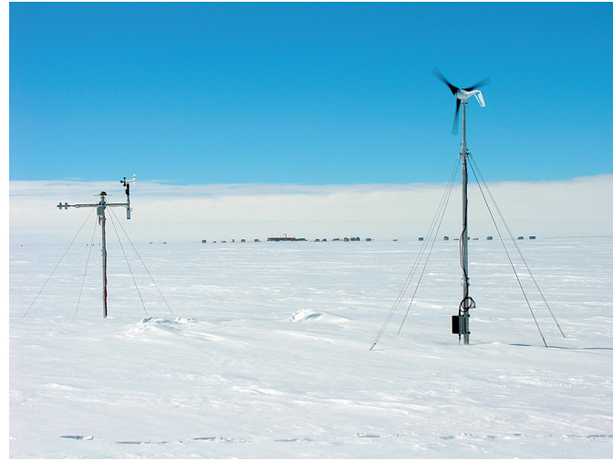
Fig. 26: The automatic weather station, AWS9, (left) at site DML05 on December 26, 2005. In 2001/02 the first station had been excavated and reconstructed approximately 150 m to the NNE of the old location (Fig. 25). In addition a wind generator (right) was installed to produce heat for the ARGOS transmitter. In the background, at a distance of 1.6 km to the east, Kohnen Station is visible. AWS9 was in operation at this site until January 2008. AWS9 belongs to University of Utrecht. (Photo H. Oerter).
