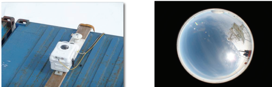
Fig. 6.1: Left: sky – imager, pyranometer and pyrgeometer mounted on top of the container on the observation deck. Right: High thin clouds near Neumayer Station with the optical appearance of a halo around the sun caused by ice particles in the higher troposphere.
