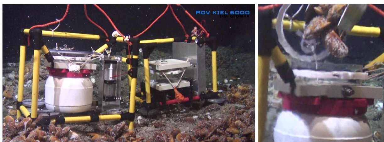
Figure 2.4.8.1: In situ fixation chambers. Left: DieFasts 1 (right) and 2 (left) sitting on the seafloor in “Clueless”. Left: Loading of mussels into a seawater-filled top chamber of DieFast 2. After closing the top lid, a trapdoor opens and the mussels slide down into the RNA Later-filled main chamber (white drum). The two-chamber design was chosen to minimize mixing of the saturated RNA Later solution with seawater during the loading with mussels.
