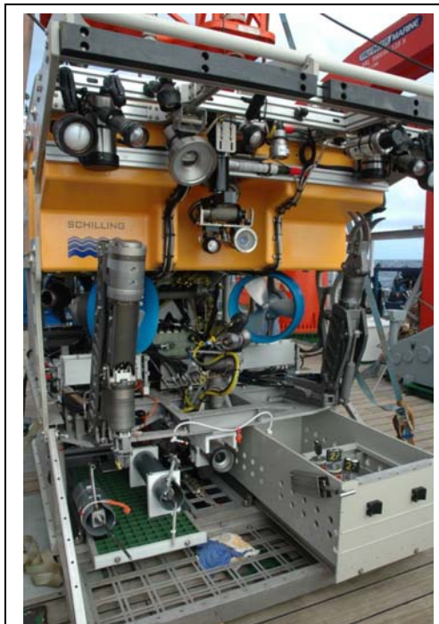
Fig. 2.4.1.1: View of the ROV Kiel 6000 front with cameras, manipulators and tool sled
