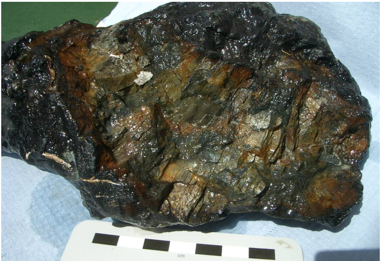
Fig. 8. Sample 310ROV-15. Serpentinite breccia; visible are cm-sized, angular, elongated, strongly sheared clasts of probably asbestos aggregates, surrounded by a black dense matrix of serpentine
