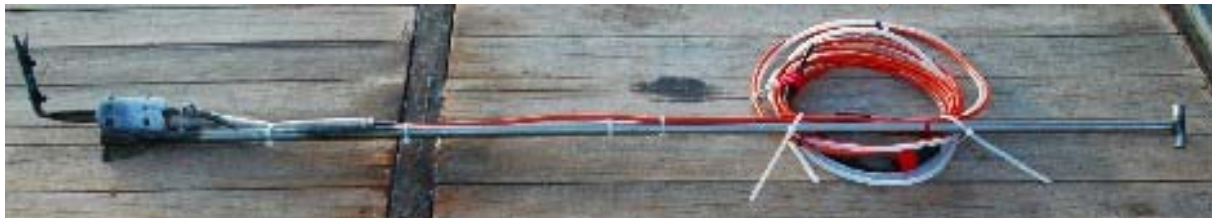
Fig. 1 T-handle extension (2 meters) with mounted KIPS Nozzle and temperature probe as used for the first sampling of the Drachenschlund vent.
