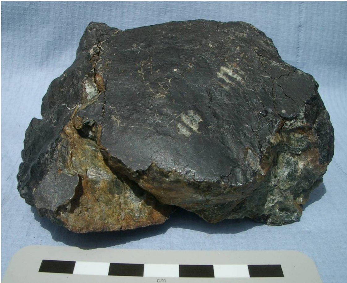
Fig. 1. Sample 310ROV-1. Tectonized microgabbro with phacoidal shape; note the strongly sheared, smooth surface.
