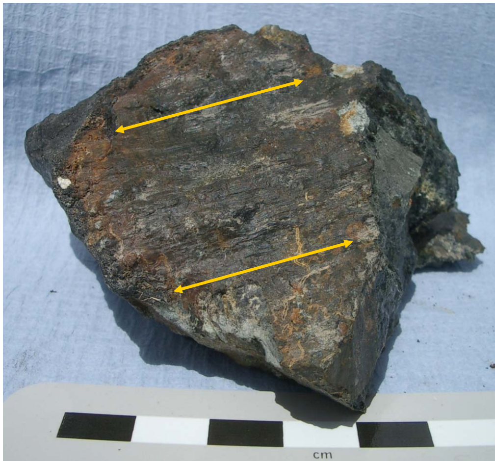
Fig. 3. Sample 310ROV-3. Serpentinite breccia with phacoidal shape; strongly sheared surface with striations (yellow arrows); sample contains angular clasts of amphibolitic ultramylonite
