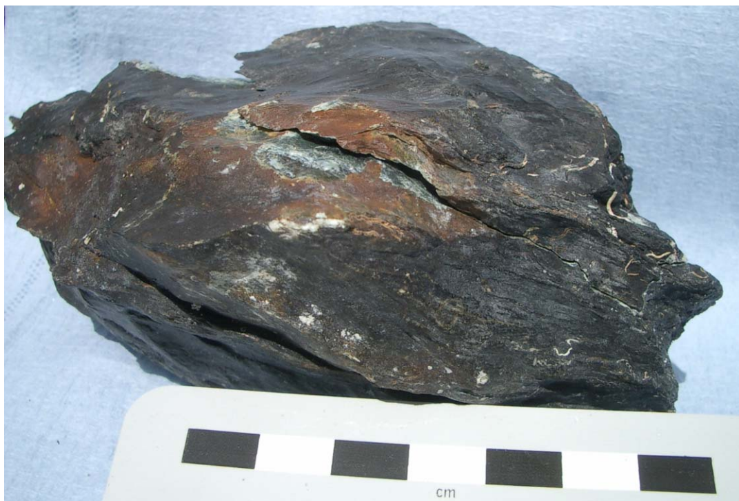
Fig. 4. Sample 310ROV-9. Serpentinite-talc schist; extremely sheared surface with striations; note that the whole sample correspond to a typical phacoid, which are visible also in the outcrop
