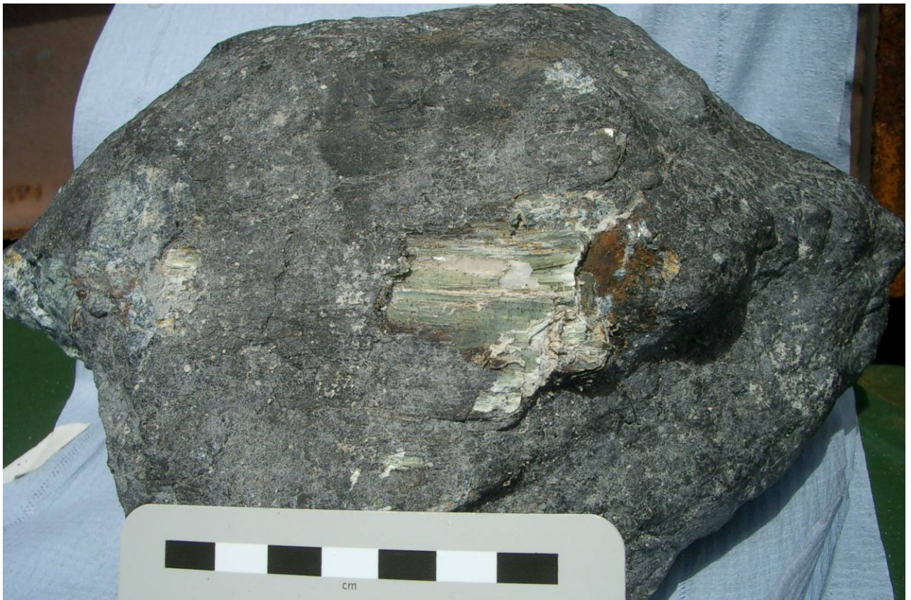
Fig. 6. Sample 310ROV-12. Sheared Serpentinite; sheared surface with striations; development of cm-sized asbestos aggregates on the surface, indicating strong shear forces at the surface
