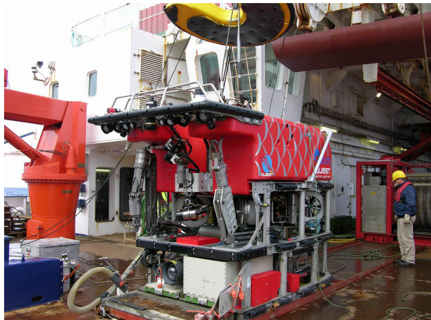
Fig. 17.2: ROV QUEST system installation aboard Polarstern (vehicle, LARS, winch, rails)
