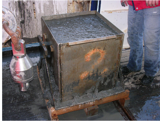
Fig. 28.3: Box corer used to sample pogonophorans
