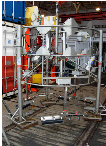
Fig. 40.1 Bottom lander equipped with sediment disturber (SD) and camera system.
