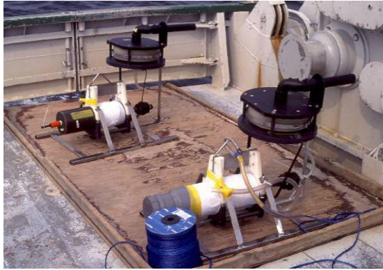
Fig. 7 Two NIOZ-SAPS systems on board RV Nereus fitted in a bottom frame as used during the spring 2007 campaign. The main body (batteries and pump) of the SAPS was placed horizontally instead of vertically while the filter unit was kept in its original (horizontal) position.
