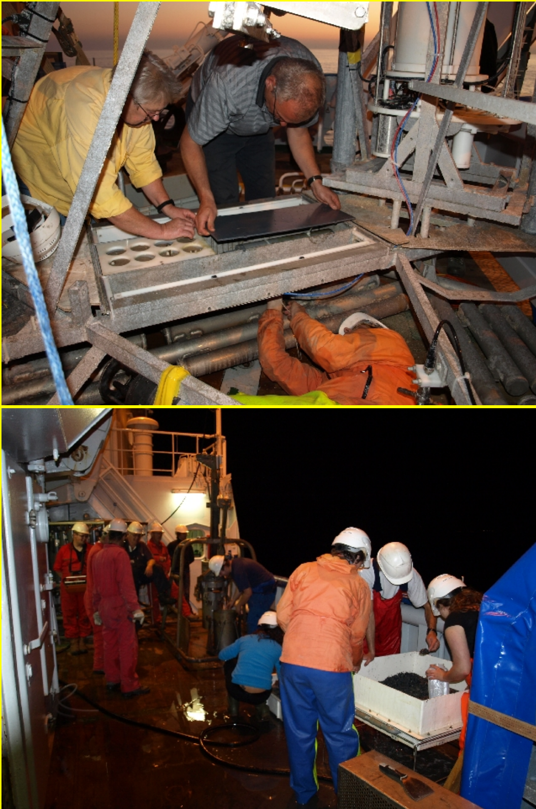
Fig. 2. The Ensis monitor is put together within the frame of the North Sea lander (Top). Boxcores are being processed on board specifically for Ensis (Bottom).
