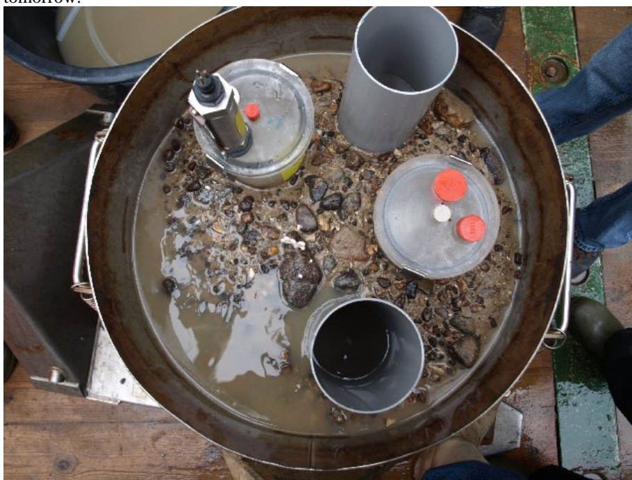
The boxcore sample full of dropstones with 2 incubation cores and the 2 geocores
