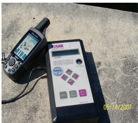
Fig. 3.3.1: To the left: GPS instrument, to the right: MICROTOPS
