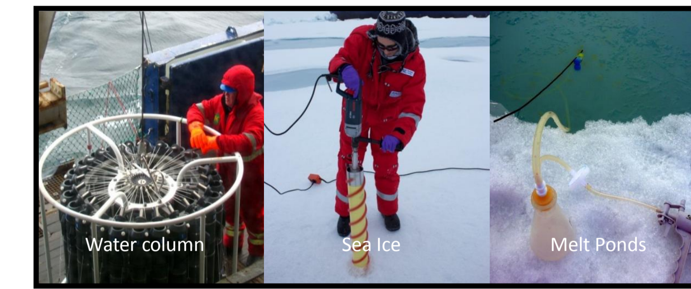
Figure 2. Sampling methods: CTD rosette, ice corer and vacuum pump.
