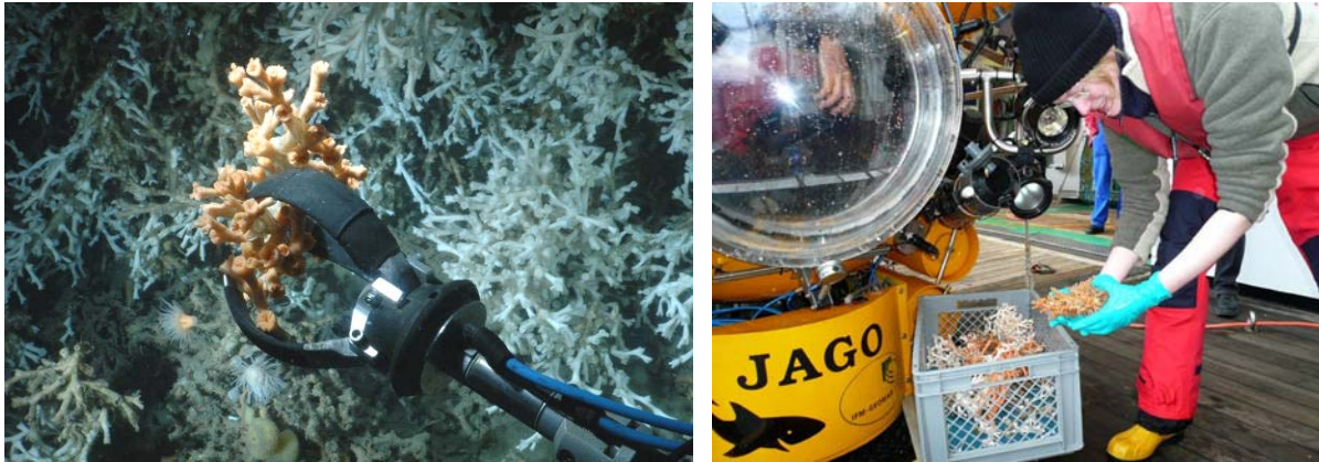
Figure 2: Selective sampling of orange Lophelia corals at Sula Ridge with the manipulator arm of research submersible JAGO at 285 m depth. Removing collected coral colonies from JAGO's sampling basket on board the RV ALKOR
