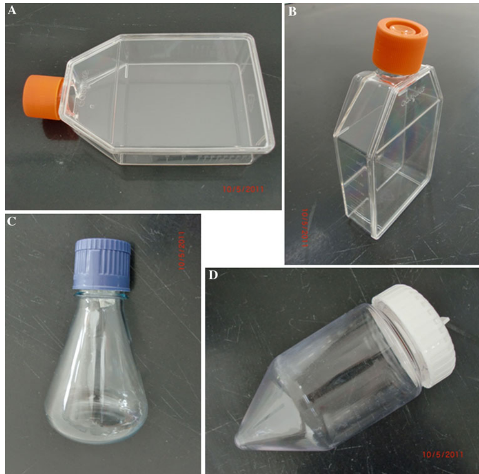
Fig. 1 Photographs of the culture flasks used in this study. a Corning culture flask (polystyrene (PS), 250 ml) horizontal position. b Corning culture flask (PS, 250 ml) vertical position. c Erlenmeyer flask (polycarbonate (PC), 250 ml). d Conical centrifuge flask horizontal position (PC, 175 ml)
