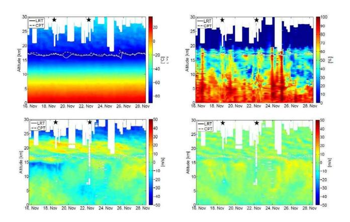
Figure 1: Profiles obtained from the radio sounding: Left: Temperature (°C), the dashed line shows the cold point temperature (CPT) and the solid line displays the lapse rate temperature (LRT); Right: Relative humidity (in %); Bottom: zonal and meridional wind components (m/s).
