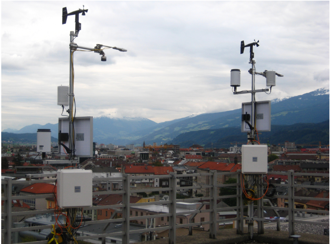
Figure 2.3: Comparing two AWS of the same type during the testing phase on the IMGI.
