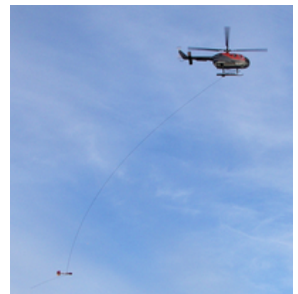
Fig. 3: The magnetic sensor is towed 30 m below the helicopter
