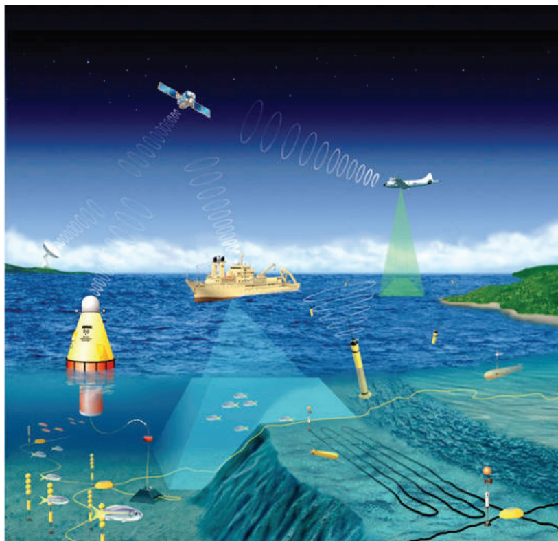
Fig. 5: Ocean observation methods include satellites, flights, commercial and research ships, surface drifters, observational platforms, tagging of animals, and robots ( http://celebrating200years.noaa.gov/visions/ioos/obs_system.html , accessed 22/09/2012).
