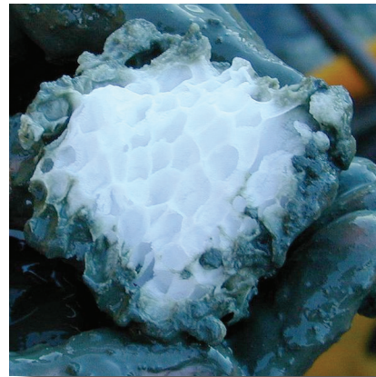
Fig. 17: Structure of a gas hydrate block embedded in the sediment. Note the cavities where the gas is held.
