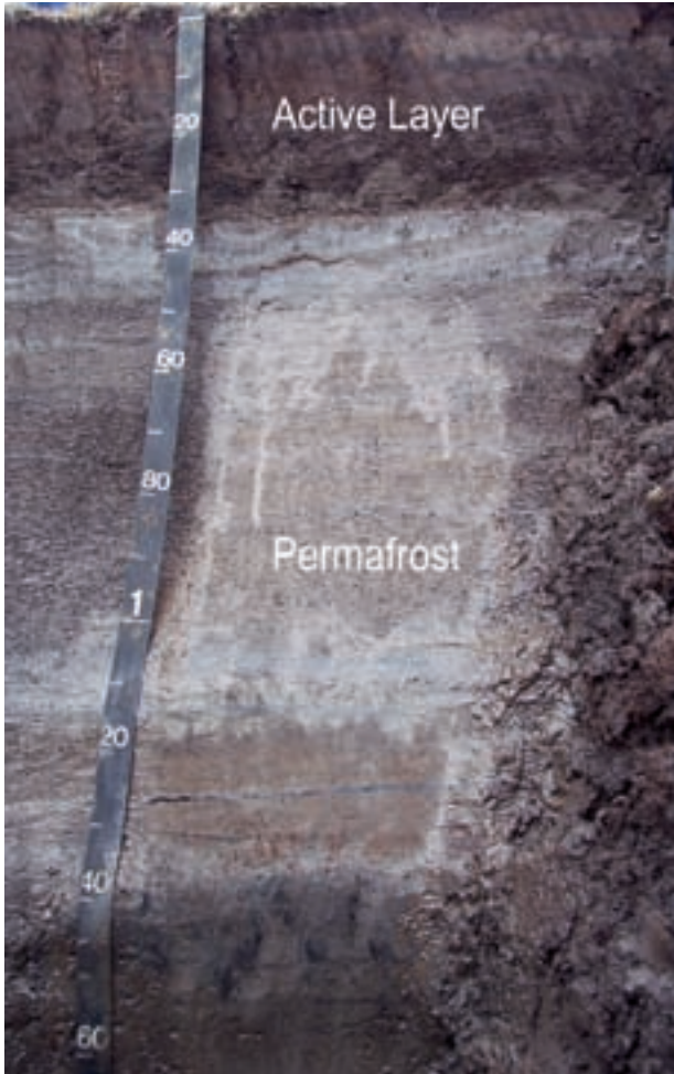
Figure 2: The thickness of the active layer at this site on the North Slope of Alaska is approximately 35 centimeters (photo: Gary Michaelson).
