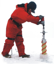
Fig. 3.1: Drilling of sea ice [credit: see list of figures].
