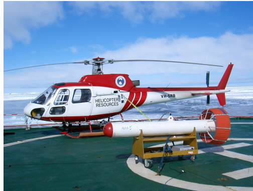
Fig. 3.5: The EM-Bird on the helicopter deck of an icebreaker [credit: A. Pfaffhuber]
