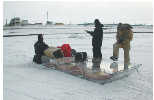
Fig. 3.2: Sledge with integrated GPR system [Holt et al. , 2009].
