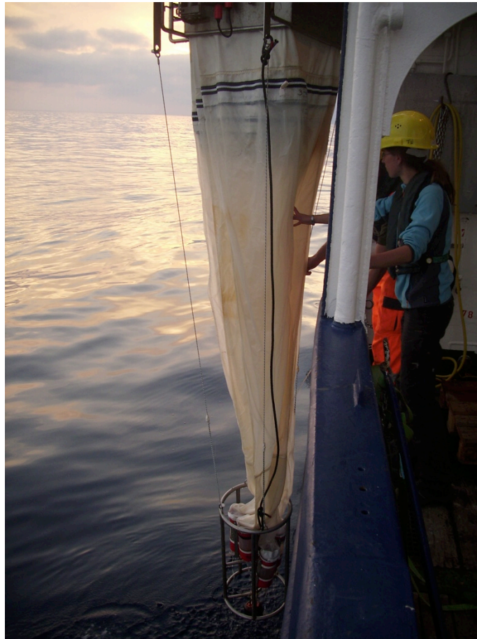
Fig. 4.2-1: The multiple closing plankton net (photo: Martin Bartels)
