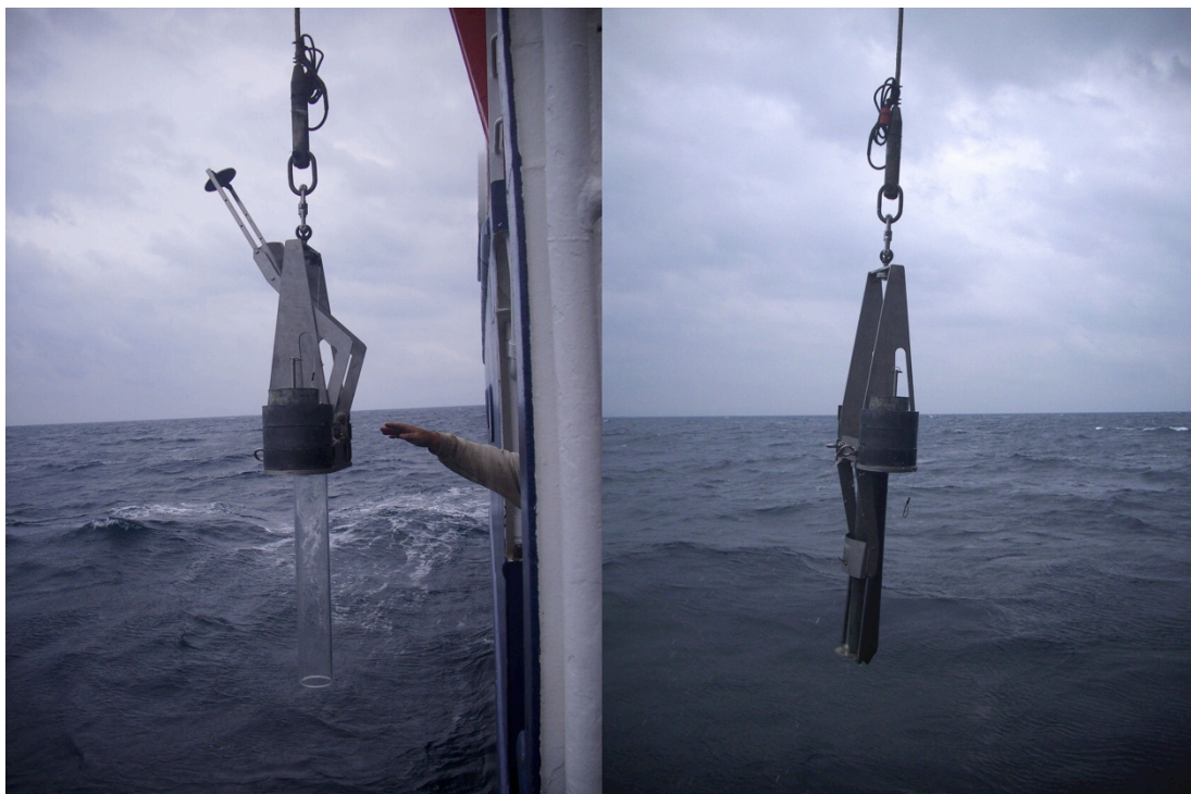
Fig. 4.4-1: Left: Frahm-corer device prepared for lowering. Right: Frahm-corer after retrieving a ~70-cm core.
