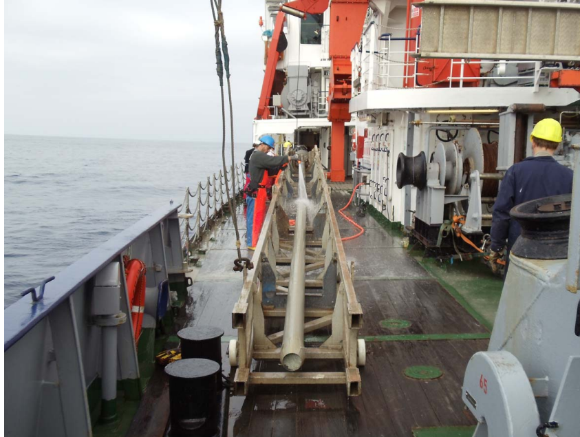
Fig. 4.4-4: Gravity cores with 12 m barrel length at station P413/4.
