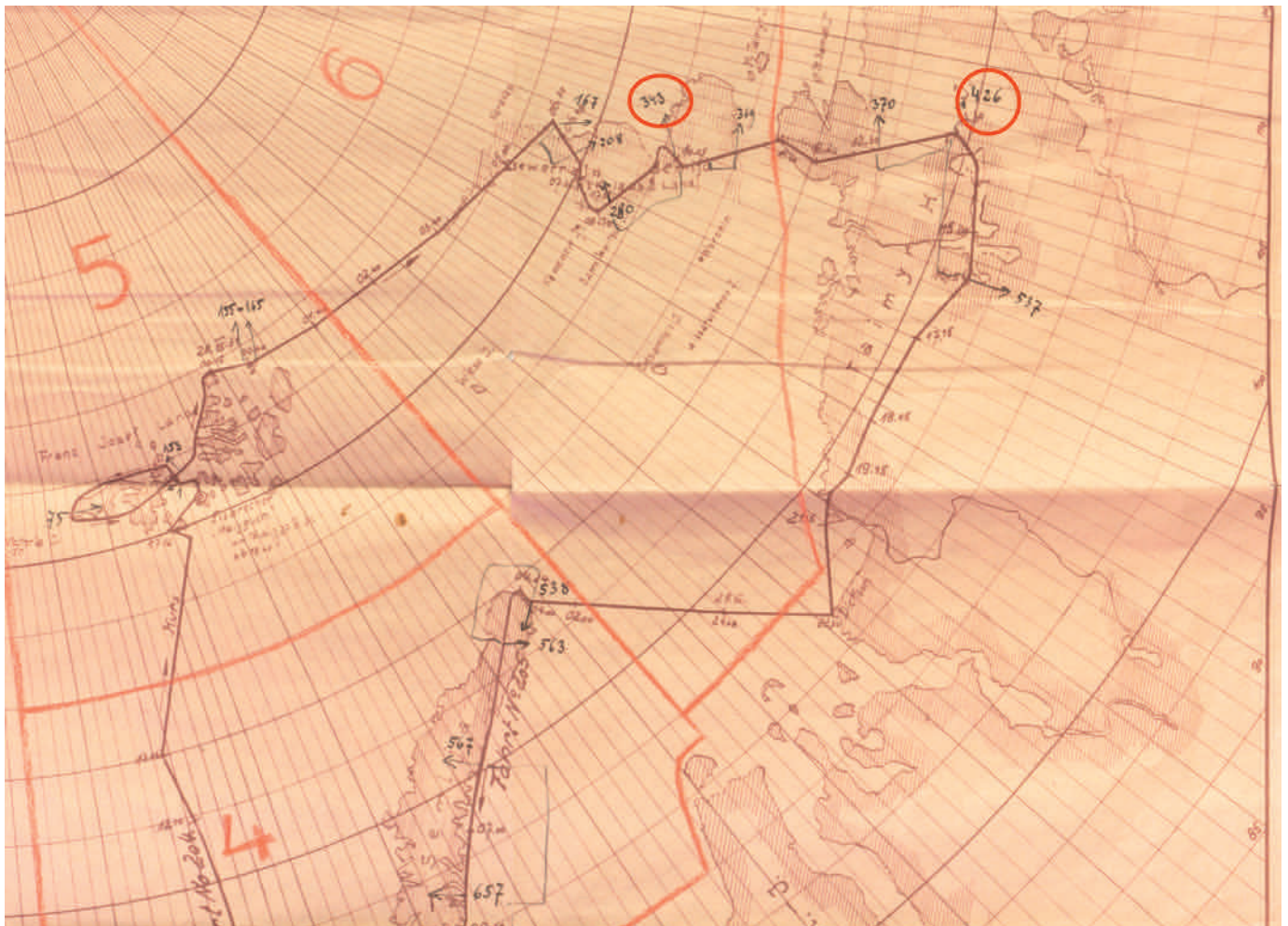
Fig. 17: Flight route of “Graf Zeppelin”, black-coloured = regions, where photos were taken with the camera type “Zweifach-Reihenmesskammer” (GRUBER v. 1931).
