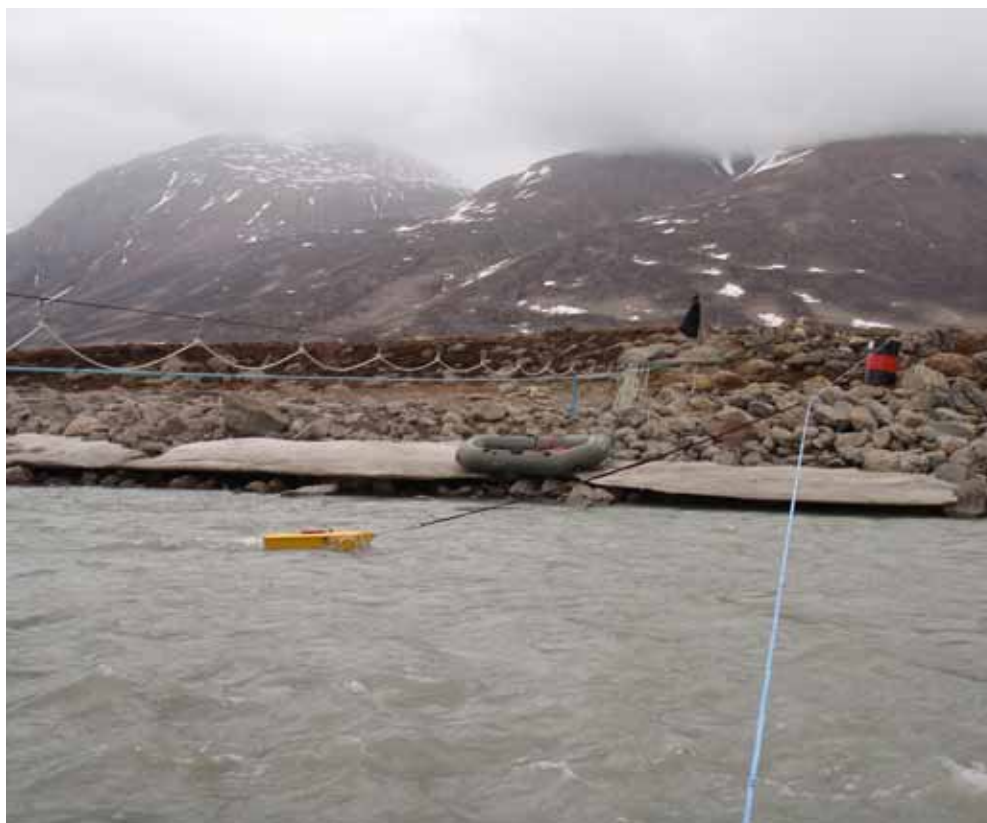
Figure 6.5 Discharge measurements with the Q-liner 22 June 2009. The Q-liner is pulled across the river with the rope and measurements at each vertical are started from land via Bluetooth communication. Photo: Kisser Thorsøe.
