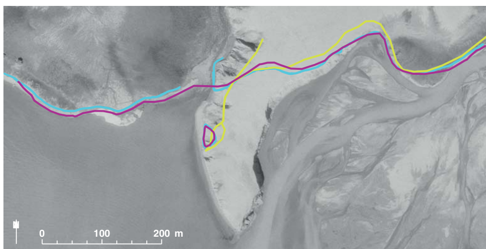
Figure 2.17 Delta and coastal cliff line measured by DGPS in 2008 (yellow line), 17 October 2010 (blue line) and 12 October 2011 (purple line) on an aerial photo from 8 August 2000.
