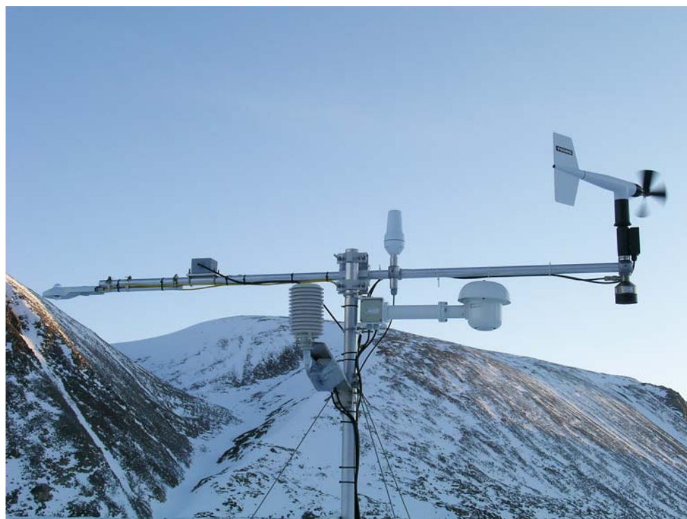
Figure 3.2 The AWS1 station in May 2011 with the addition of a Vaisala passive radiation shield for comparison with the standard Rotronics aspirated shield. Photo: Signe Hillerup Larsen, GEUS.
