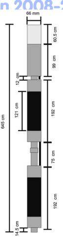
*Fig.* 1 - Simplified diagram of the downhole hydraulic fracturing tool and straddle packer assembly.
