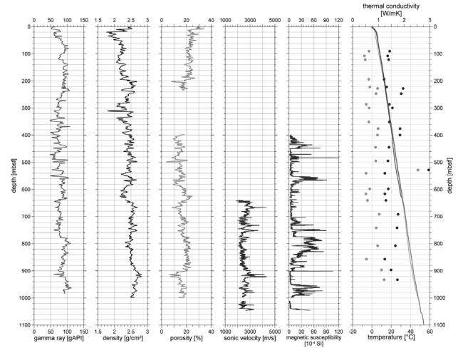
*Fig.* 4 – Most important downhole logging data of the Southern McMurdo Sound Project, AND-2A borehole: gamma-ray, density, neutron porosity, sonic velocity, magnetic susceptibility, and temperature. Some lab-originated thermal conductivity measurements on plugs are added (light dots - dry samples; solid dots - water-saturated samples).
