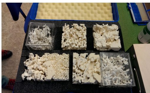
Christoph Mitterer explaining the metamorphism of snow using hands-on models of the pore space obtained from micro-computer tomography (Photos: O. Eisen)
