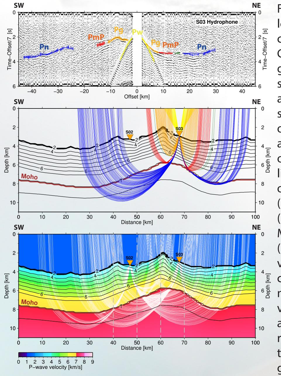
For the wide-angle seismic survey a cluster of four G-gun type airguns was used as seismic sources average and an shot point spacing of 150m was Results achieved. of forward modeling and inversion of refracted crustal and mantle (Pq) phases and (Pn) reflected Moho (PmP) phases provide a 2D image of crustal and upper mantle P-wave velocities. High amplitude crustal refractions indicate steep velocity gradients near the
